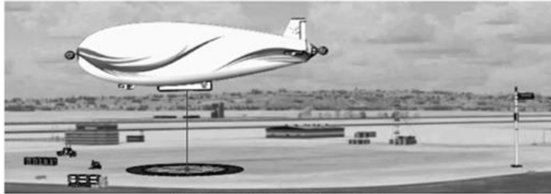
Mooring the airship MB 310 using winches
