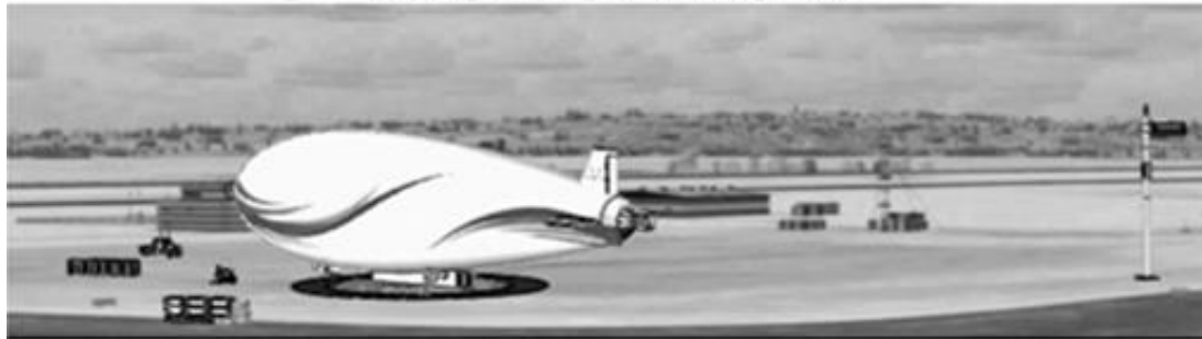
Rotating the turntable to point airship's nose in the direction of wind
